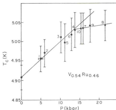
FIG. 4. Pressure dependence of  $T_c$  for  $V_{0.54}Ru_{0.46}$ .
